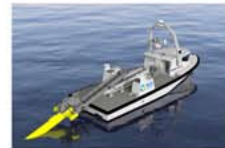
INSPECTOR 125 Carrying a mid-size AUV or various towed SAS / SSS with its LARS
